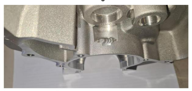
Spindle on both sides of crankcase. area for crankwebs Ø93mm area for con rod Ø95mm
