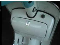
If the box doesn't fit perfectly to the legshield, you can grind it's edge down to match. Mount with the rubber trim and you're done.
