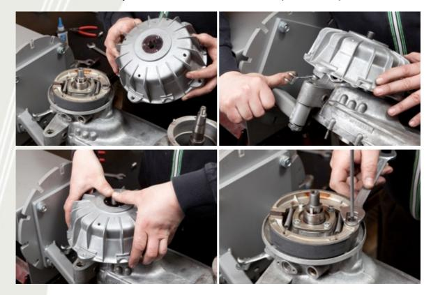
Step 5: When the settings are done, the hub can be fully fitted. Make sure you are using the wavy washer under The domed nut and also apply some Loctite to the allen screw holding the lock washer.
