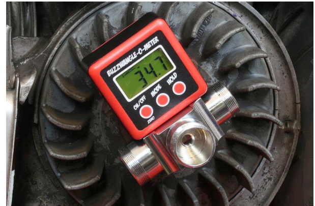
The Buzzwangle-O-Meter will read crankshaft rotation from any zeroed position
