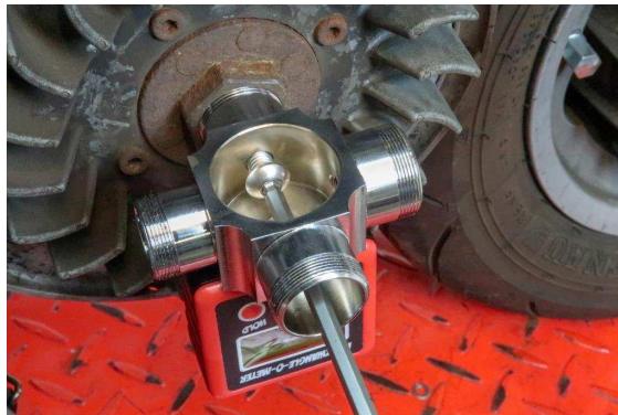
Tighten the Allen screw against the crankshaft to lock the Buzzwangle in any position.
