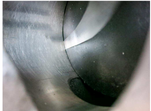
A thin feeler gauge trapped in the port by the piston crown.
