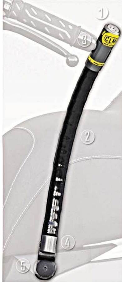
2. Internal Steel cable of 5 millimeter diameter resistant to more than one ton traction protected for mechanized joints of hardened steel of 1,5 mm thick.
