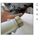
Once your hands are greasy smear the exhaust adaptor bush and the connection of U-bend and main box. This makes un-assembling at later stages very easy and prevents the parts sticking together forever.
