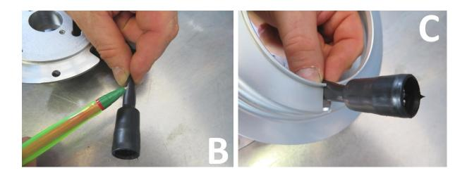
Gently squash the wires inside the sleeving at the point seen in **Pic. B**, so that they are in line. Now insert the sleeving into the slot of the backplate, right through to the main exit hole as seen in **Pic.C**, keeping the wires in line whilst doing so.
