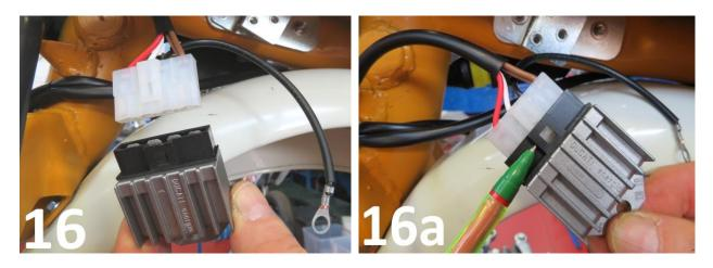
16) Insert the plug-in connector for the voltage regulator into its socket, ensuring that the retaining lug is fully seated home, as per **Pics 16 + 16a.**
