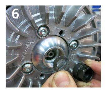
6) Fit the washer and the nut to the crankshaft, as per Pic. 6. Remember this has a left-hand thread!
