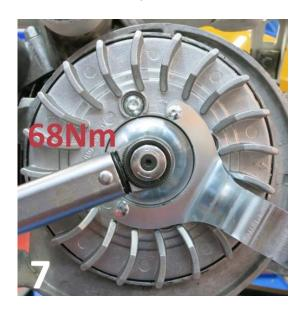
7) Using the special tool to block the flywheel, tighten the nut to <u>68Nm (50lbs-ft)</u>, as per Pic. 7.
