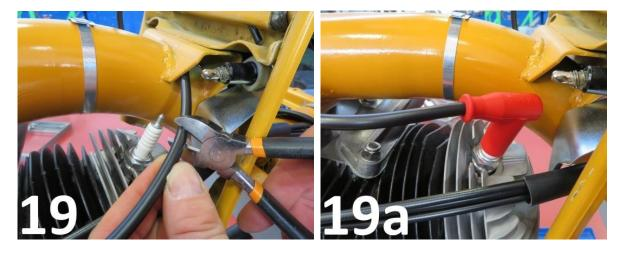
19) Pass the HT lead along the desired routing of your scooter and cut it to length, allowing a little excess for suspension movement. Fit the spark plug cap. See **Pics. 19 + 19a.**
