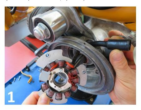
1) Insert stator plate wiring through the hole in the magneto flange as per Pic. 1.
