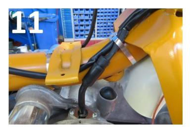
11) Clamp the wiring harness to the scooter's frame. Leave the wiring from the magneto flange slightly curved, with a little excess in length to allow for suspension movement, as per **Pic. 11.**
