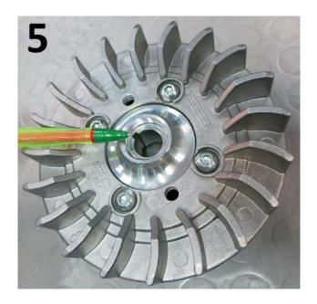
5) The woodruff key must be aligned with the recess in the flywheel as indicated in **Pic. 5** when inserting the flywheel onto the crankshaft taper.
