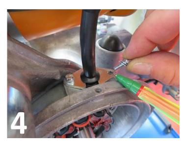
4) Fix the plate to the magneto housing using the original 4mm screws and washers as per **Pic. 4**.
