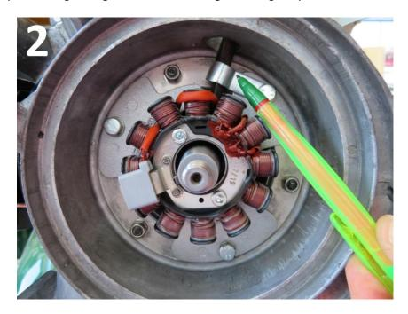
2) Fix the stator plate using the original 3 bolts and washers. Attention must be given to the wiring retaining plate to ensure that it does not damage the sleeving. See **Pic. 2.**
