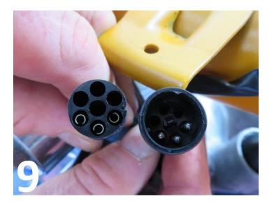
9) The round connector plug from the stator plate has corresponding holes for the pins of the supplied wiring harness, as can be seen in **Pic. 9.** There is also a groove external recess so it is literally impossible to misalign.
