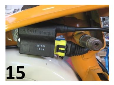
15) Mount the CDI to its brackets using the supplied 5mm bolts and washers, as per **Pic 15**. This type of CDI does not have an external earth wire. *This is easier to do with the rear supension unit removed.*
