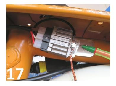
17) Mount the Voltage regulator to its brackets using the supplied 5mm bolt and washer, as per **Pic 17**. This bolt can also accommodate the earth wires from both the voltage regulator and the braided earth wire that connects to the flywheel cowling.
