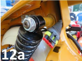
12) Pass the plug-in connector for the CDI between the top of the main frame tube and the metal plate that supports the seat crest pressing. See **Pics. 12 + 12a**. If the connector cannot physically pass between the main tube and the flat plate (as there are variations between some Lambretta models), pass it over the top through to the other side and then slide the wiring down into the gap. *There may be some differences between Lambretta models*.
