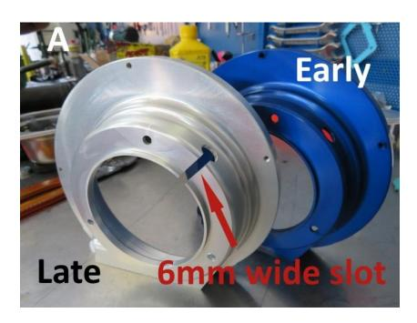
You need to remove the backplate from your engine and make a 6mm wide slot as indicated in **Pic. A.** The slot must be cut from the existing hole inwards, towards the centre of the large central aperture. All current production backplates for **CasaCase** engines and **CasaCooler** magneto flange kits now have this slot incorporated as standard.
