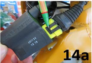
14) Insert the plug-in connector for the CDI into its socket, ensuring that the retaining clip is fully seated home, as per **Pics. 14 + 14a**.
