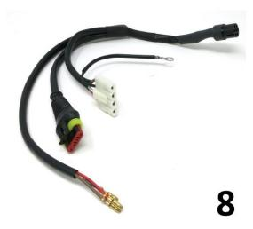
8) The **Casatronic Ducati** igntion comes supplied with a separate, small wiring harness with simple, push-in waterproof connectors to connect up the stator plate directly to both the regulator and the CDI unit.
