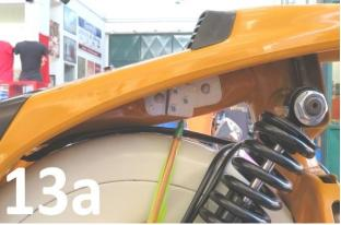
13) Fit the 2 brackets for mounting the CDI and the Voltage regulator to the frame, as per **Pics. 13 + 13a.** The 2 brackets are identical and must be mounted as per the pics. At the time of writing (August 2019), currently supplied brackets are solely for Series 3 machines. Designated brackets for Series 1 + 2 machines will be available shortly.
