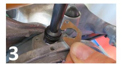
3) Insert the LT wires fixing plate into the grooved recess of the rubber bung as per Pic. 3.
