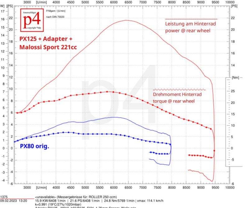
Adapter PX125 - M210, h60/P125, SI24, 1.75mm Spacer, Welle orig
