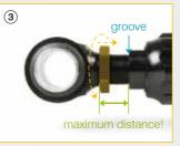
3) groove has to be covered completely in shocker mainbody
