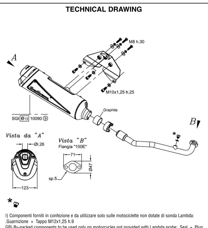
GB) By-packed components to be used only on motorcycles not provided with Lambda probe: .Seal + Plug M12x1,25 h.9
